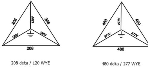
Figure 3: AC grids supported by SolarEdge three-phase inverters
