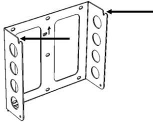
Figure 13: Bracket with U-shaped indentations facing up
