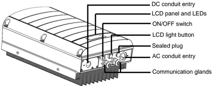
**Figure 9: Inverter connectors (single phase example)**
