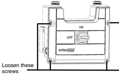
**Figure 11: Opening the AC/DC Safety Switch cover**
