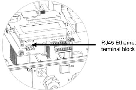
Figure 28: The RJ45 Ethernet connector
