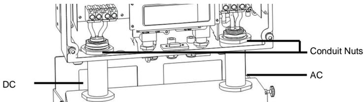
Figure 44: Inserting the AC and DC conduits
