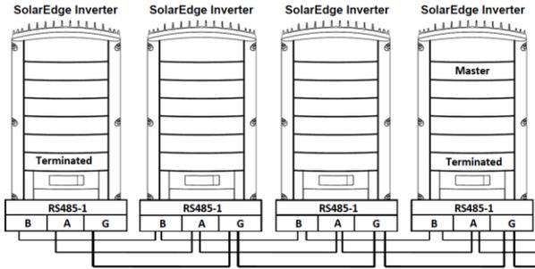
Figure 31: Connecting the Inverters in a Chain
