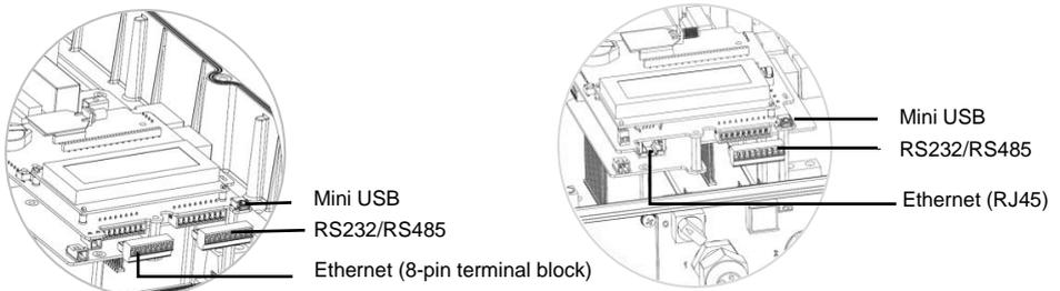
Figure 24: Internal connectors
