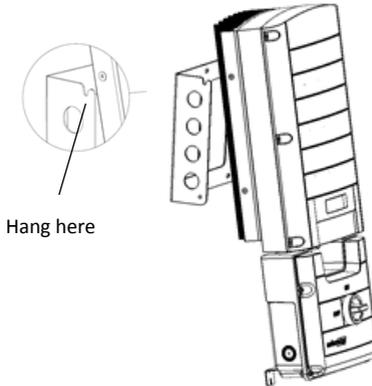
Figure 14: Hanging the inverter on the bracket
