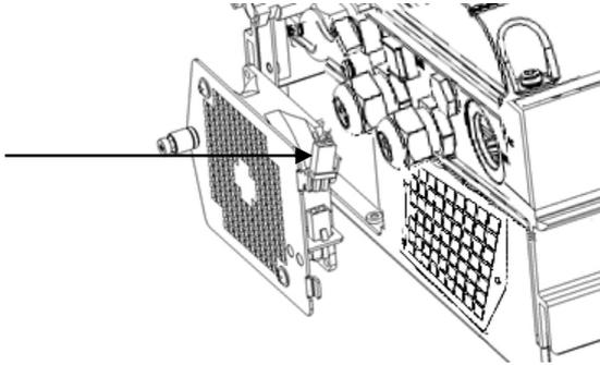
**Figure 43: Fan connector**
