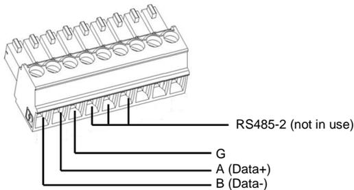
Figure 30: RS485/RS232 terminal block
